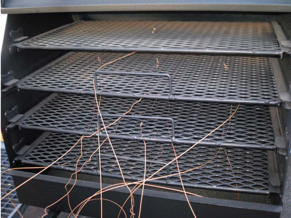
Figure 3. A view of a partial installation thermocouples. All wires are then ported out to the front bottom of the lid.
